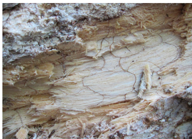
Fig. 3. Well developed white rot with conspicuous brown lines.
